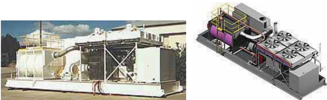
Figure 2.1 Photographic Views of Tomlinson Inert Gas Generator (after Tomlinson Boilers, 2004)
