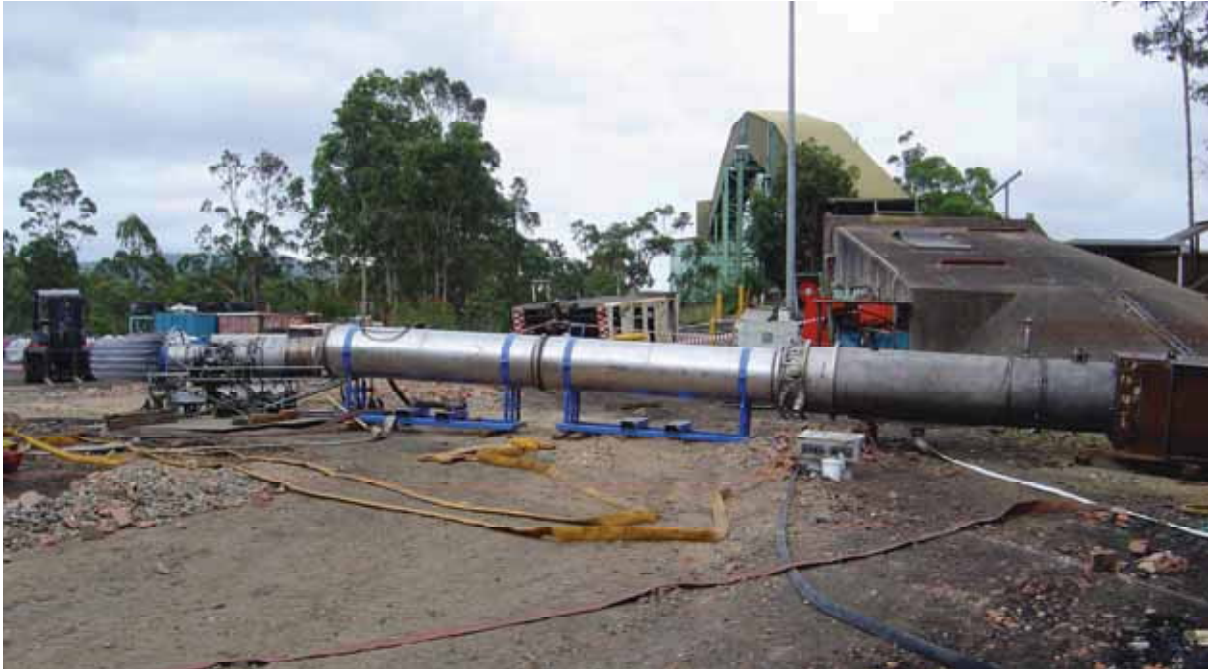
Figure 2.17 GAG 3A Jet Engine set up at Southland Colliery, 2003
