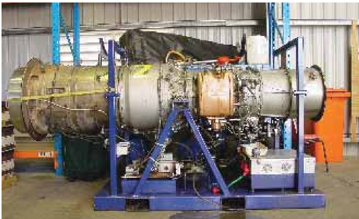
Figure 2.6 One of the Queensland Mines Rescue Service GAG-3A inertisation units
